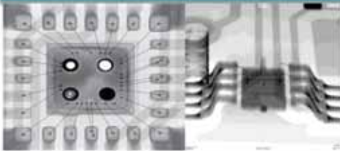
Inspection of Wire Bonding in IC
